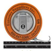
Figure 3: Diameter tape used for the inventory
