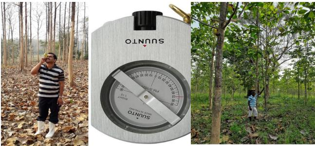
**Figure 4:** Total Tree height was measured by hypsometer and a pole, used instrument of sununto meter is shown in above
